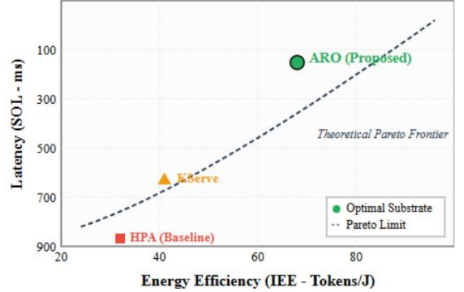
Figure 3. Multi-objective optimization frontier for distributed LLM inference. The chart illustrates the Pareto dominance of ARO over reactive baselines (HPA, KServe) in minimizing scheduling latency while maximizing tokens-per-joule efficiency.
